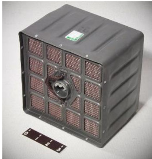
Figure 1: Lithium Hydroxide Cannister [3]
