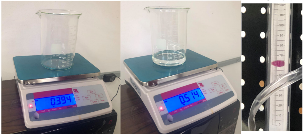
Figure 28 Weighing water to find volume, comparing to output of flow meter
