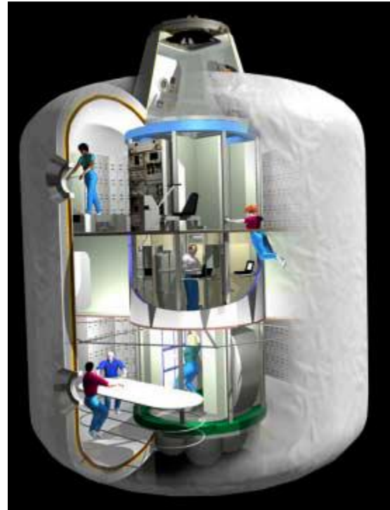
Figure 3. Vertical Orientation of TransHab
