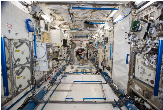
Figure 2. Foot Rails and Handrails Aboard the ISS
