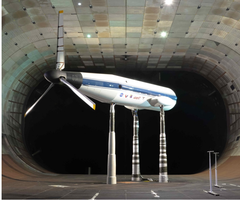
Fig. 1. TTR/699 installed in the NFAC 40x80 test section (the TTR is oriented at 45° yaw).
