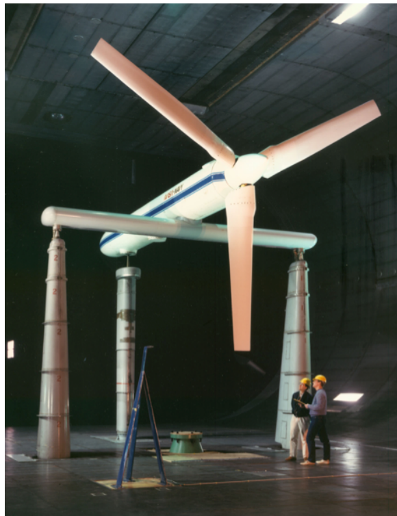
Fig. 32. Scaled JVX rotor on the Prop Test Rig (1991).
