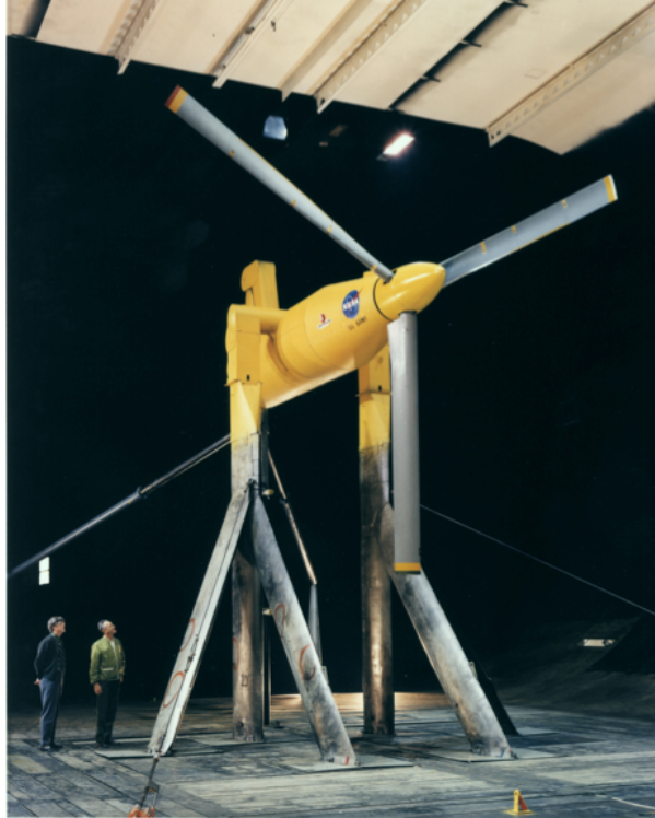
Fig. 31. XV-15 rotor on the Propeller Test Rig (1970).
