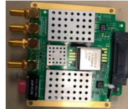
NC3m GNSS RF card(~3.5"x3.5")
