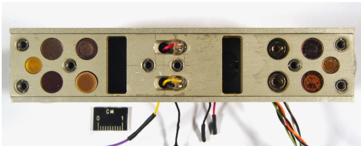
Figure 19. Post-flight photograph with the lid removed and the passive samples and ram facing photodiodes visible.
