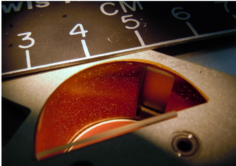
Figure 22. Post-flight photograph of the passive scatterometer chamber showing salt remaining on the Kapton liner.
