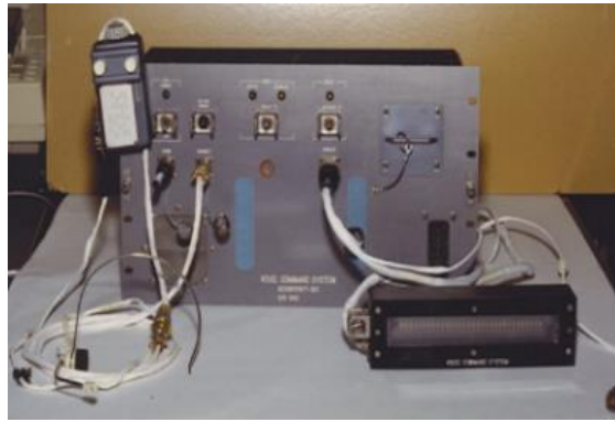
Figure 4. Voice Command System Hardware Components (Credit: NASA)
