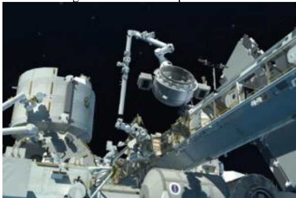
Fig. 14. The Nanoracks Bishop Airlock can be opened to space to release satellites and run experiments. It can also be detached and moved to different locations. Taking advantage of the opportunity to expose experiments to different elements such as sunlight or atomic oxygen, this flexibility enables a wide range of research possibilities. Credits: Nanoracks
