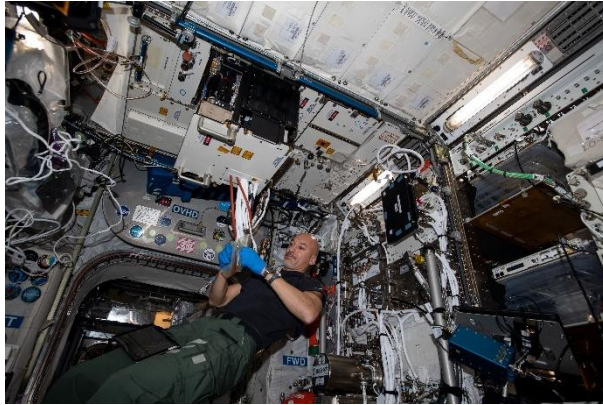
Fig. 13. ESA astronaut Luca Parmitano installing the MultiScale Boiling Experiment Container (EC) in the Fluid Science Laboratory (FSL) in the Columbus Module aboard the ISS. Credits: NASA/ESA
