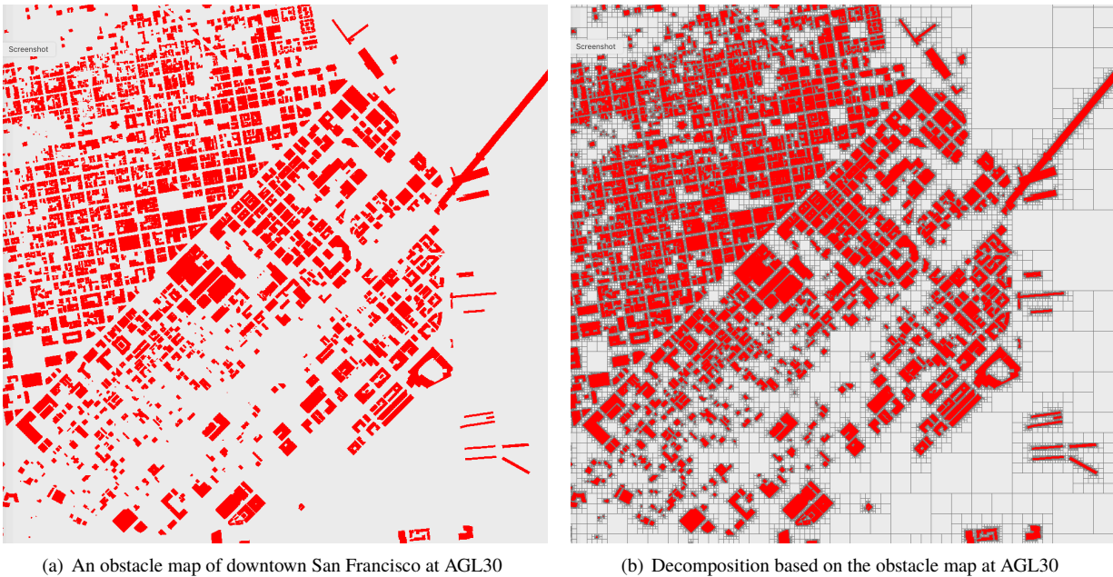
Fig. 4 Obstacle map and its quad-tree decomposition for downtown San Francisco at AGL30
