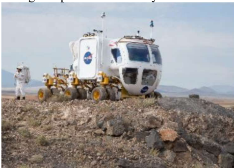
Figure 1. Pressurized rover prototype testing at the Black Point Lava Flow near Flagstaff, Arizona.
