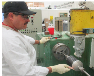
Commercial Scale CNT Composite Winding
