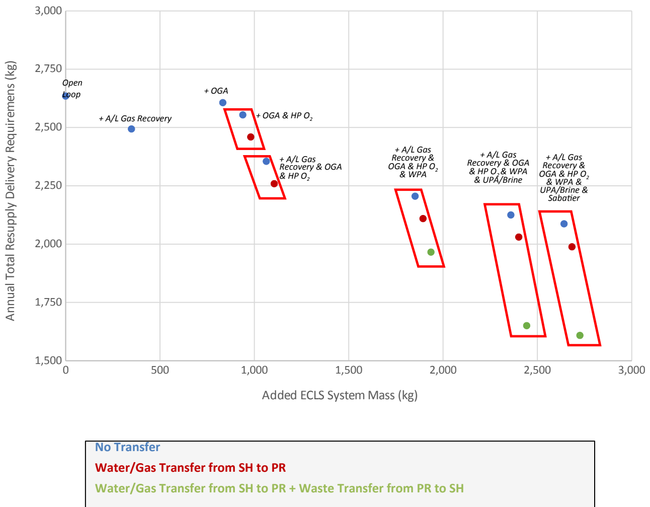
Figure 3. Annual Outyear Logistics vs Added ECLSS Mass – Grouped by Regenerative ECLSS Capability
