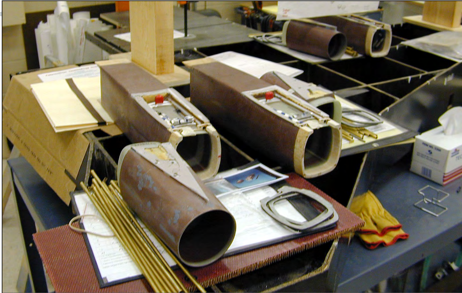
Completed Engine Inlets and Nozzles
