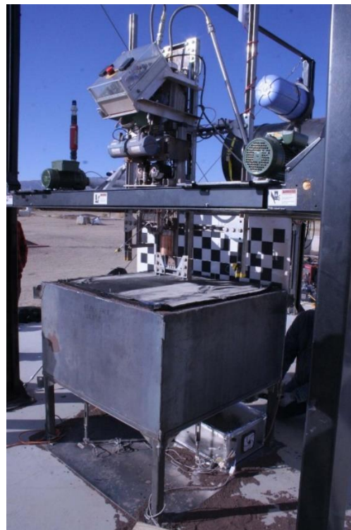
Figure 4. Test stand regolith container with a test material installed.
