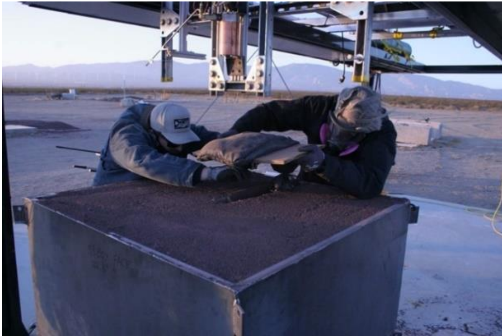
Figure 2. Regolith-filled steel box used under engine for landing pad materials test showing instrumentation as it is being installed
