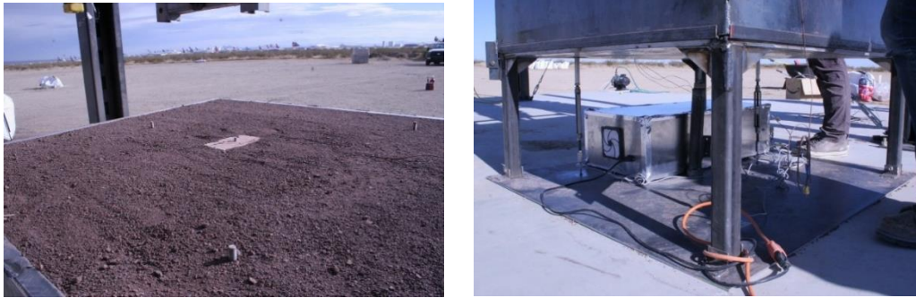
Figure 6. Threaded rod interfaces to the load cells at the top of the regolith surface (left). Configuration of the turnbuckles and load cells below the regolith box alongside the DAQ enclosure (right)
