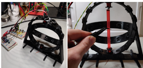
Fig. 4 Early Reaction Sphere Levitation Test Rig
