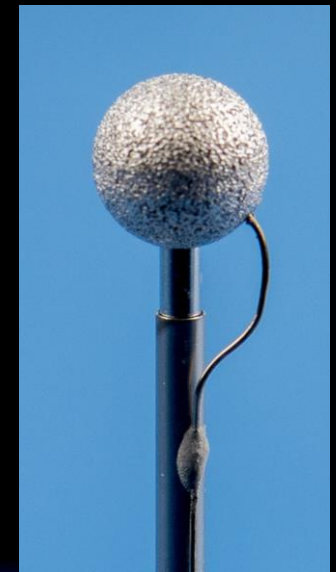
6.35-mm porous spherical burner
