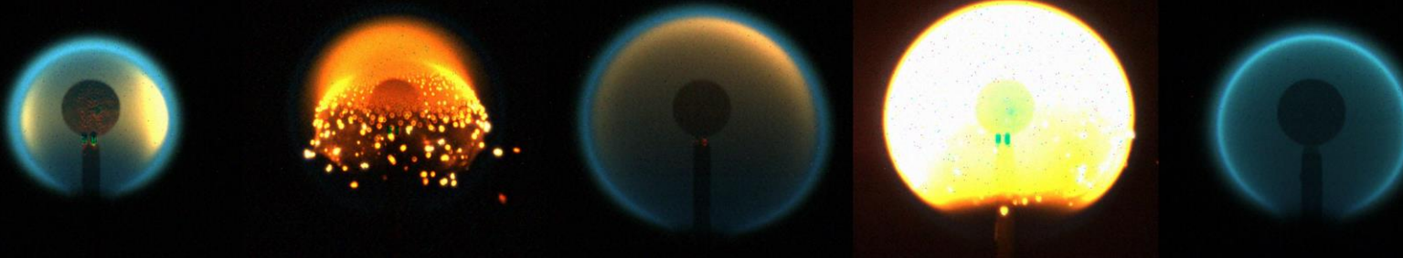
Flames with a variety of sooting characteristics
