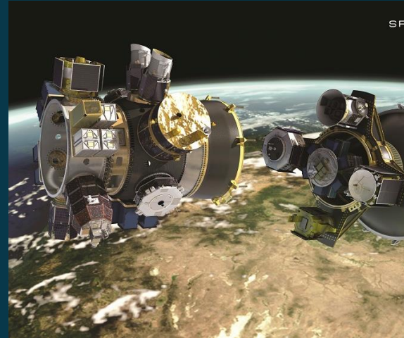
ESPA-Ring Payload Port Limit (450 kg)
