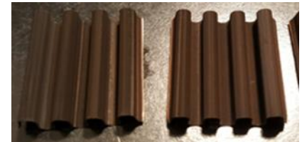
Laser processed CHX fins (FLSP on complex surfaces)
