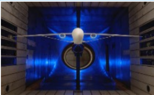
Transonic Truss-Braced Wing 5-10% fuel burn benefit
