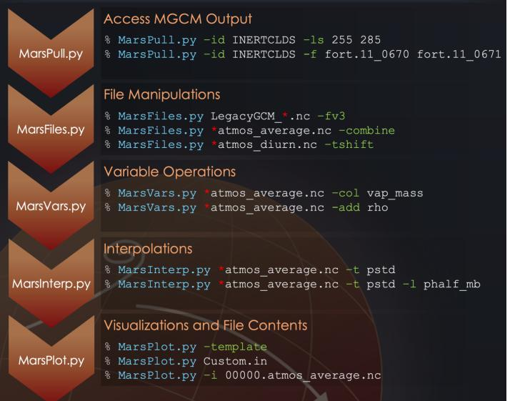
CAP is designed to be modular. For example, a user could post-process and plot MGCM output exclusively with CAP or a user could employ their own post-processing routine and then use CAP to plot the data. Users are free to selectively integrate CAP into their own analysis routine to the extent they see fit.
