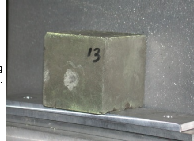
Sulfur cement/regolith blend following impact testing. Image credit: NASA.
