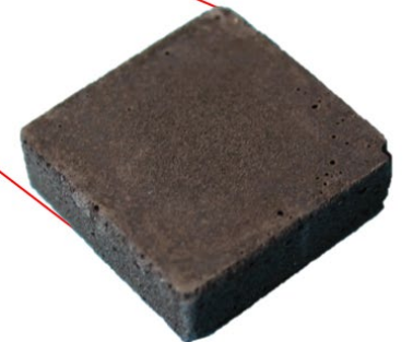
Materials ISS Experiment 15 contains multiple geopolymer samples. Image of geopolymer square courtesy of Penn State/Peter Collins and Aleksandra Radlinska.
