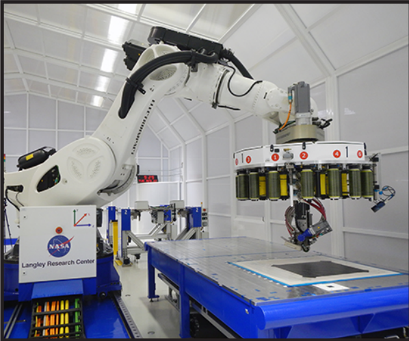
Fabrication of a carbon-epoxy panel using AFP on ISAAC
