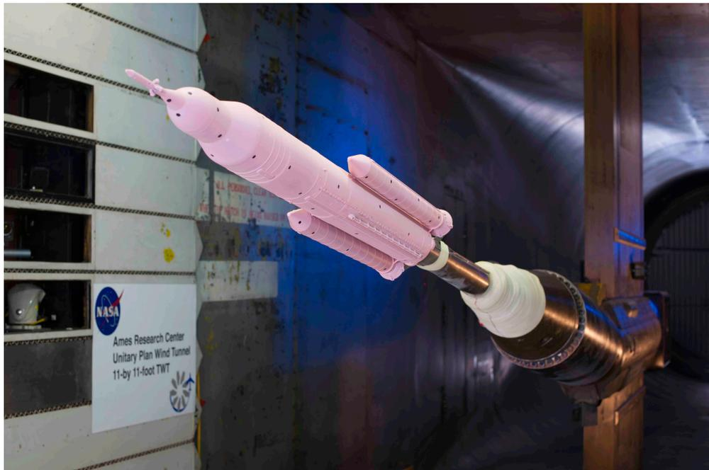
**Fig. 3** SLS Block 1B Crew model with PSP applied to model in the NASA ARC 11-Ft TWT.
