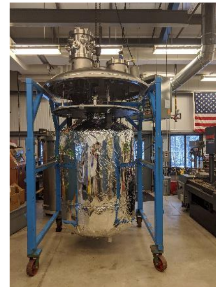
Prototype Test Article with MLI
