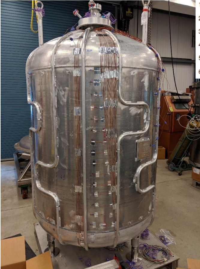
Prototype Test Tank before and after insulation installation.
