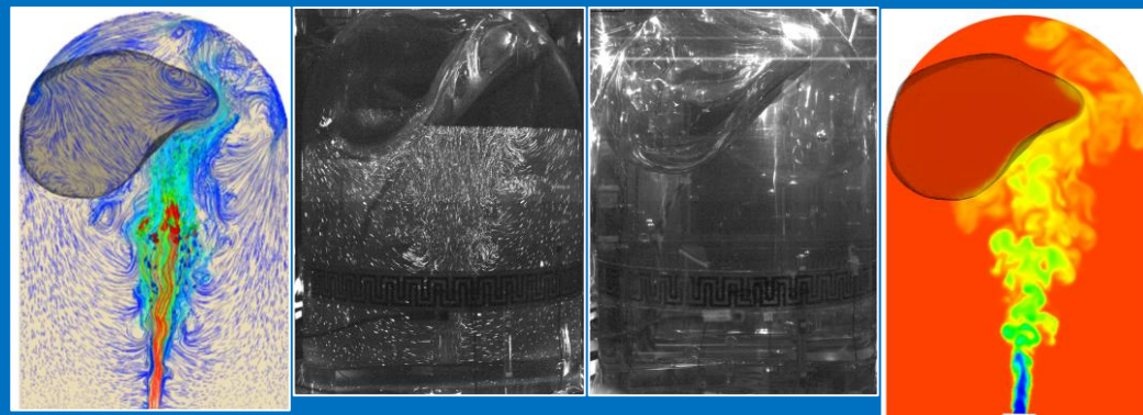
Non-intuitive Microgravity Jet Ullage Interaction & Current Validated CFD Model Predictions
