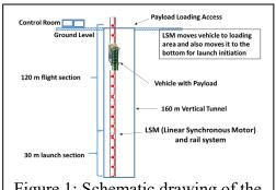
Figure 1: Schematic drawing of the proposed ElectroMotive Drop Tower
