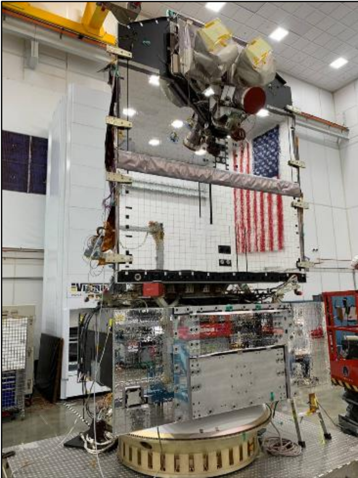
LCRD payload (top) integrated onto STPSat-6 space vehicle, July 2020 Credits: NASA
