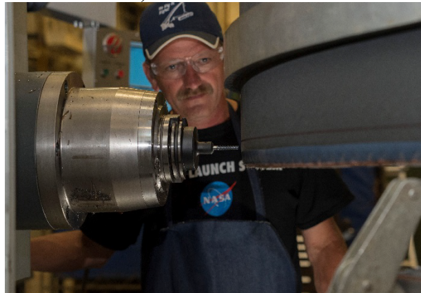
f) Trimming and machining holes in the areas of the load introduction fixtures.
