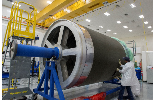
b) Manual adhesive film and honeycomb core application.
