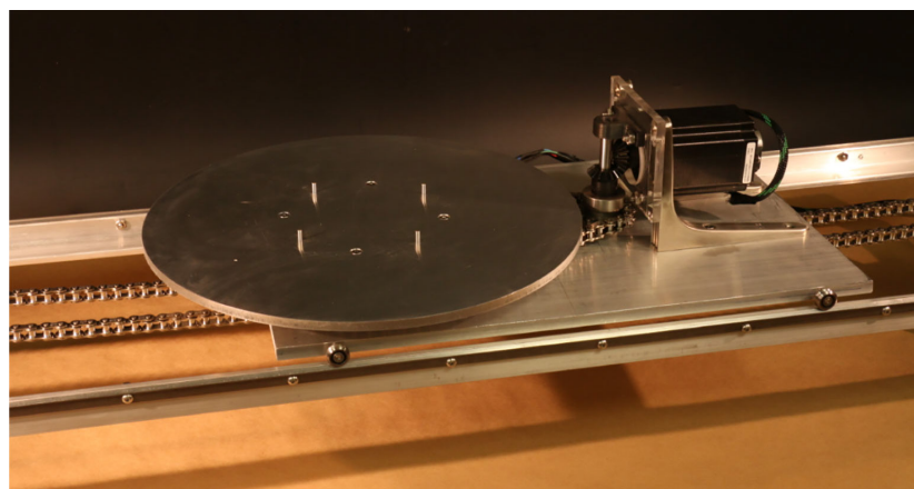
Figure 6.—Spin plate installed on carriage on transfer rails.
