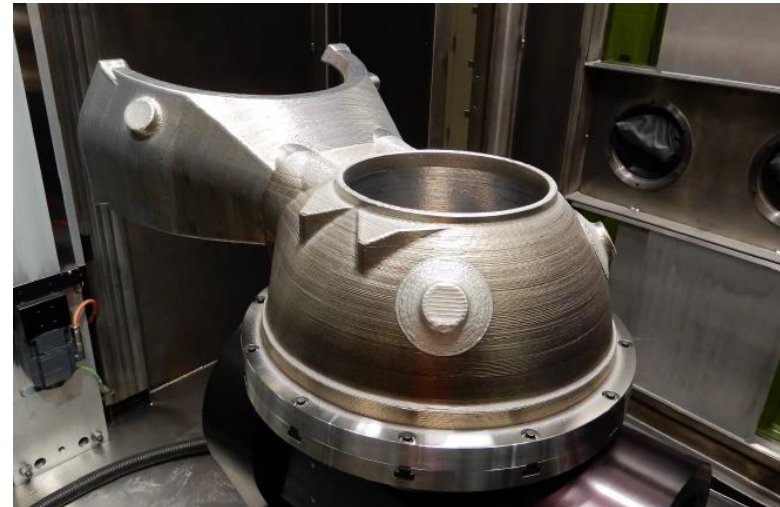
RS25 Powerhead demonstrator using LP-DED under NASA SLS Artemis Program (Courtesy: RPMI)
