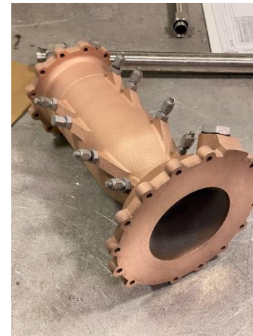
L-PBF GRCop-42 Combustion Chamber, NASA HR-1 LP-DED Nozzle, Inconel 625 L-PBF Injector
