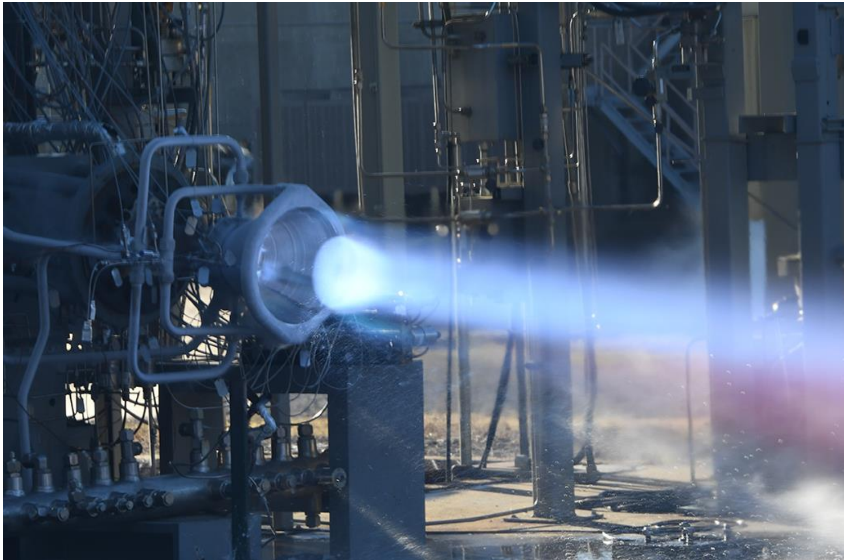
L-PBF GRCop-42 Combustion Chamber, NASA HR-1 LP-DED Nozzle, Inconel 625 L-PBF Injector
