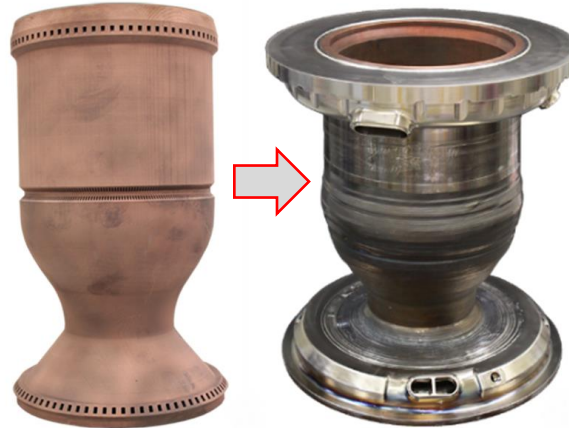
EB-DED Inco 625 Jacket on L-PBF GRCop-84 Liner
