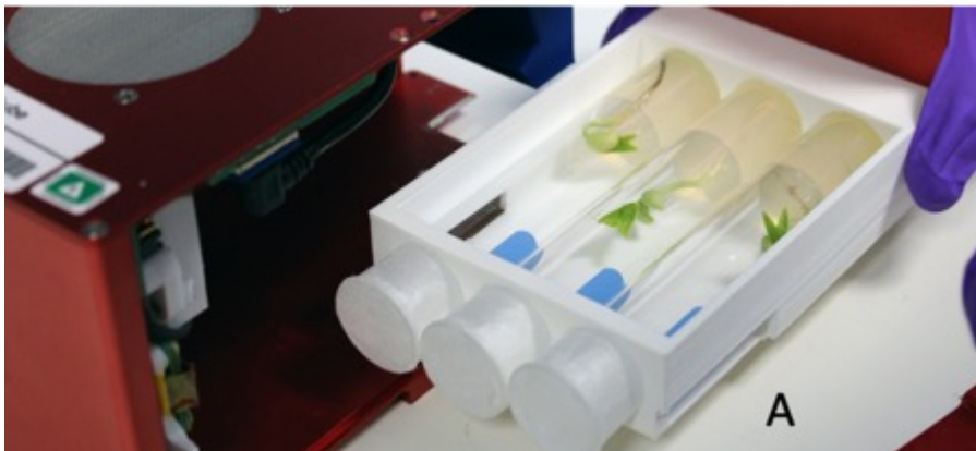
(A) 2U CubeLab growth chamber installation. (B) Malting CubeLab investigation with fluid and thermal control subsystems. (C) On-Orbit plant growth image.
