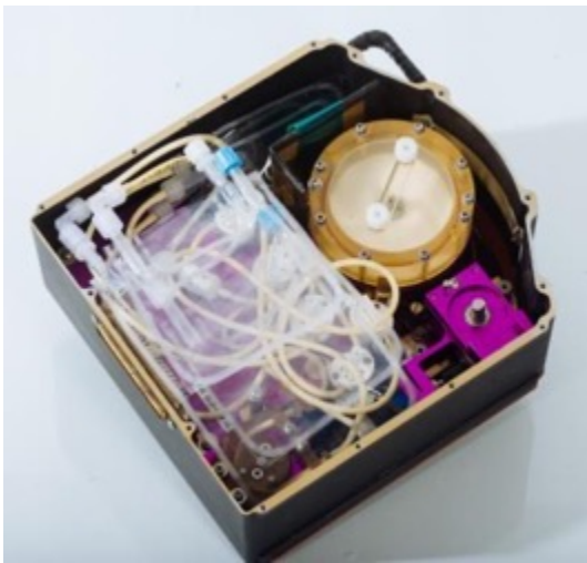
Cell Culturing: 50 ml rotating bioreactor, automated feeding, waste & sample collection and fixing.
