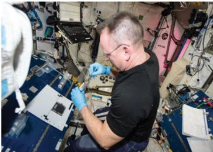
Astronaut Butch Wilmore fixing plants on ISS using a K ennedy F ixation T ube (KFT).
