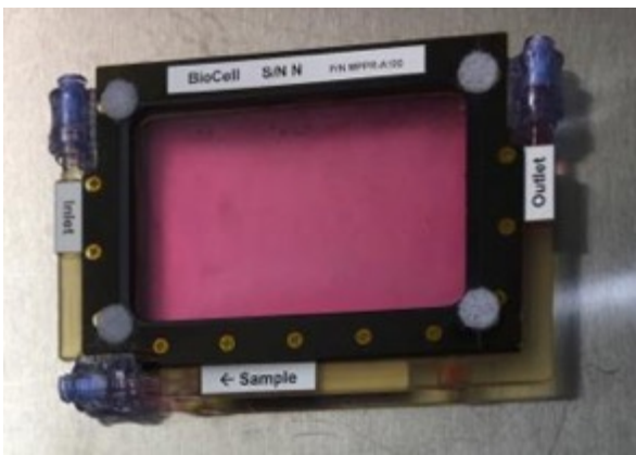
Single-Well BioCell filled with Growth Medium.
