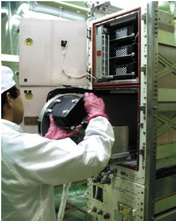
CBEF open showing \mu G Compartment (top) and 1G Compartment (bottom).
