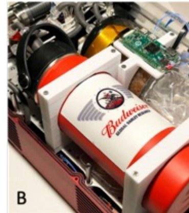
(A) 2U CubeLab growth chamber installation. (B) Malting CubeLab investigation with fluid and thermal control subsystems. (C) On-Orbit plant growth image.
