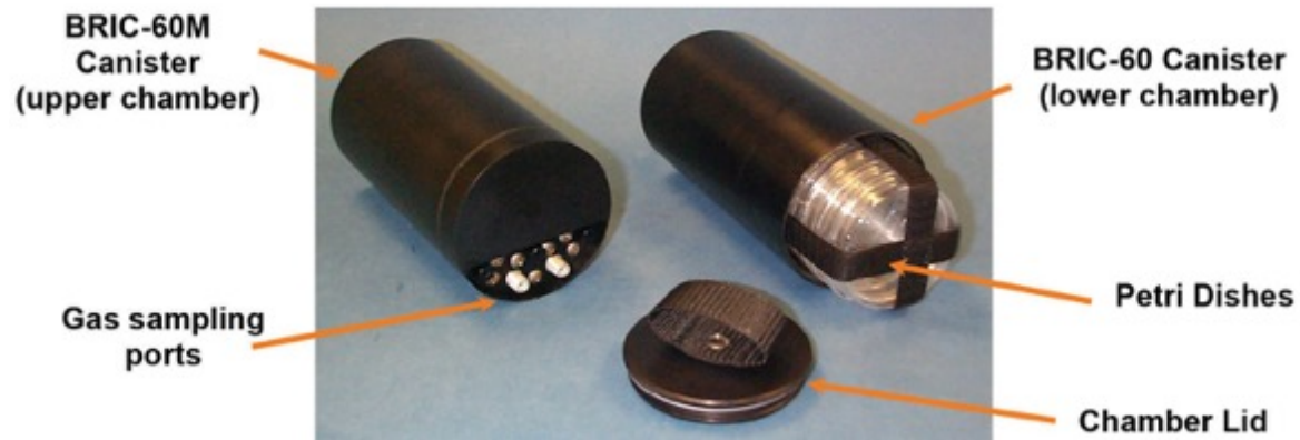
Fig. 1. BRIC-60 & BRIC-60M with petri dish configuration. Teflon sample tubes.
