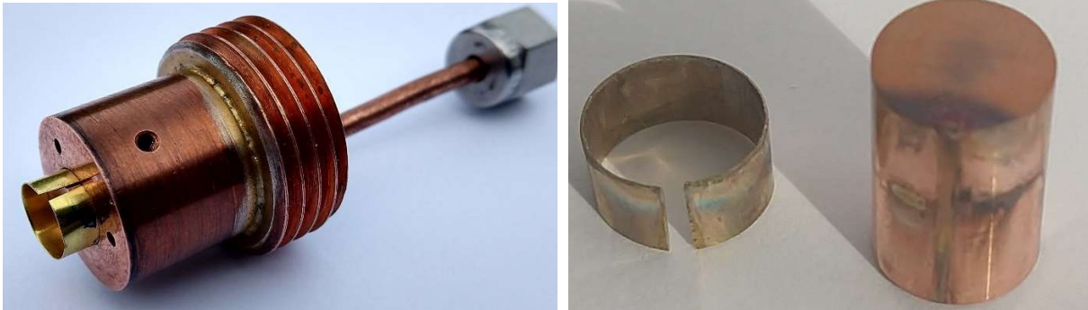
Fig 7. a) Slug Calorimeter with brass shim stock partially inserted into the gap. b) post-test discoloration
