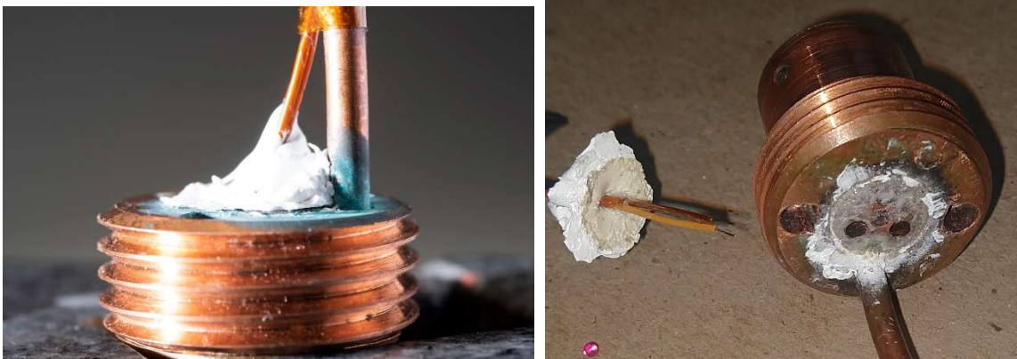
Fig. 11 Slug holder backside with Ceramabond sealant that has debonded
