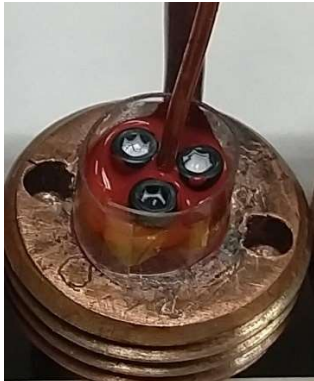
Fig. 13 a) Slug holder with RTV sealant b) Heat flux measurement with and without RTV
