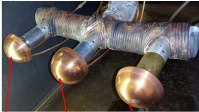
Fig 15 a) Coaxial TC probes mounted on a trident b) Radial distribution of heating measured by probes 9 & 10
