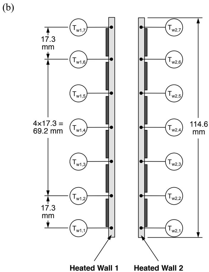
**Fig. 1** Schematic representations of (a) overall construction of Flow Boiling Module (FBM), (b) construction of heating slabs, and (c) substrate temperature measurement.
