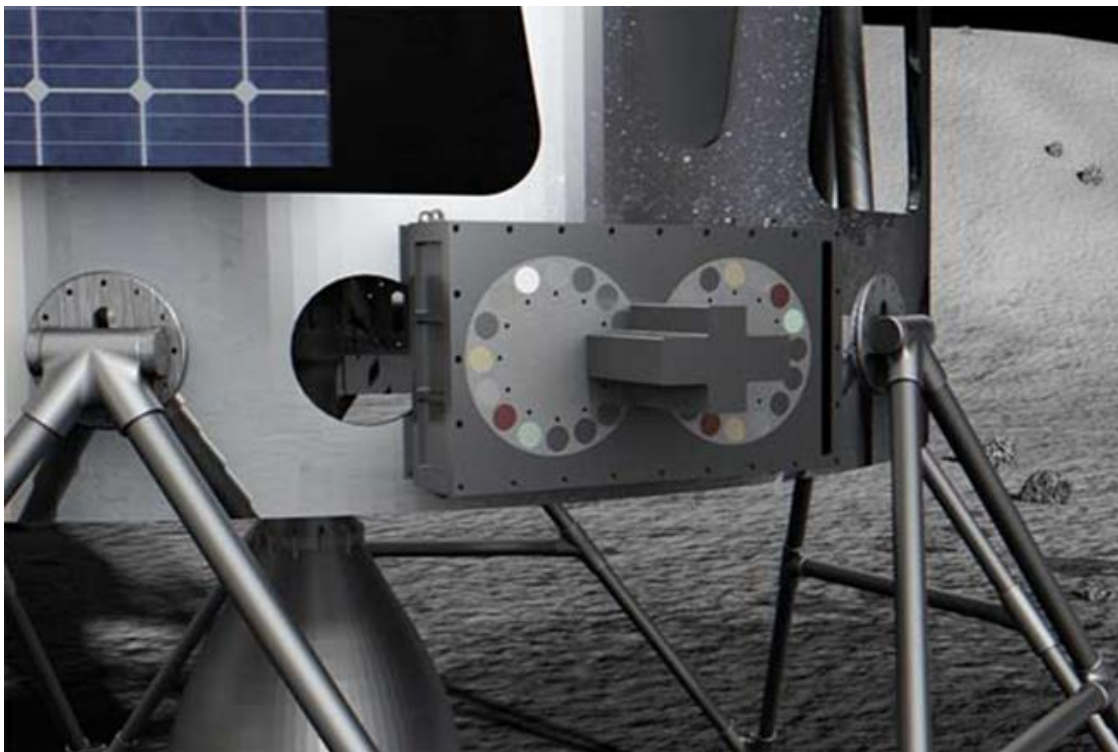
Figure 1. Schematic of the Regolith Adherence Characterization (RAC) payload being provided by Alpha Space Test and Research Alliance, LLC. Image credit: Alpha Space Test and Research Alliance, LLC.
