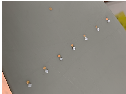
Figure 7. Trips applied to model; 0.56 mm height (and 1.3 mm width) trips shown.
