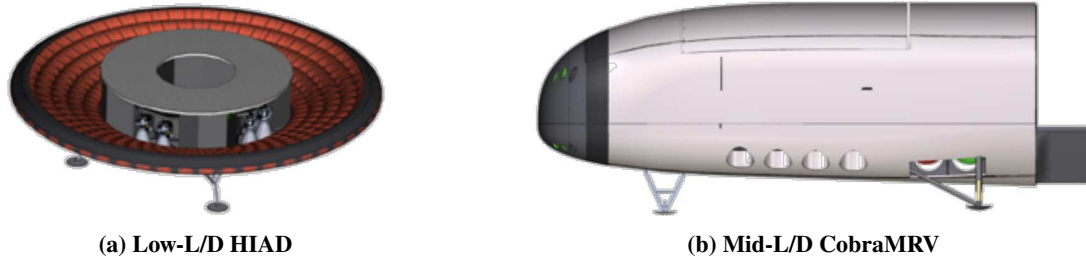
Fig. 1 Concept Mars EDL vehicles for human exploration missions [1]
