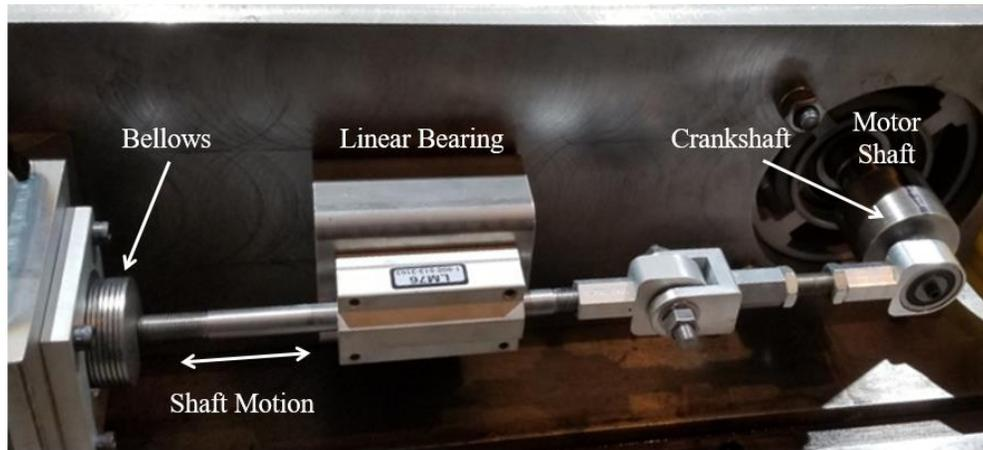
**Fig. 19 – Fatigue tester with short bellows prototype**
