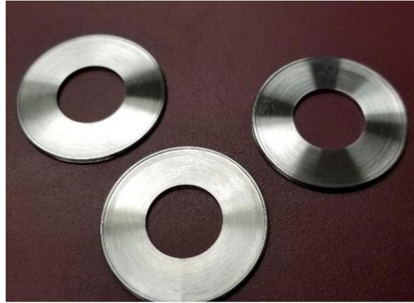
**Fig.16 Individual convolutions prior to outer diameter weld**
