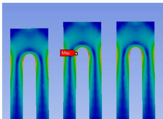
**Fig. 13 Detail of maximum stress location on inner diameter slot**
