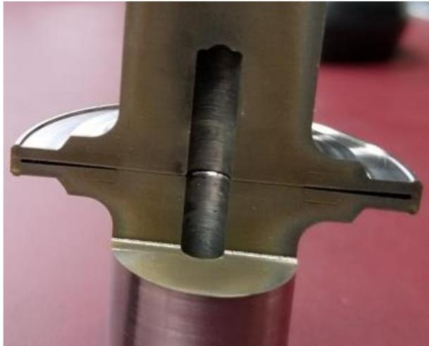
**Fig. 17 Cross section of test article for weld pull test**
