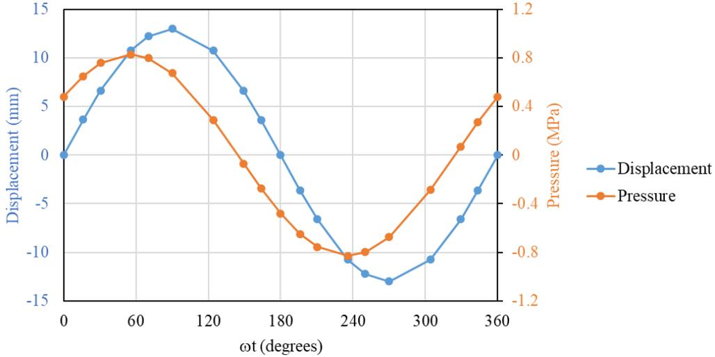
**Fig. 4 Displacement of and pressure differential across bellows**
