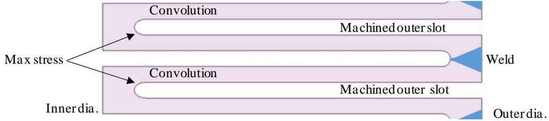
**Fig. 6 Bellows with convolutions welded at outer diameter**
