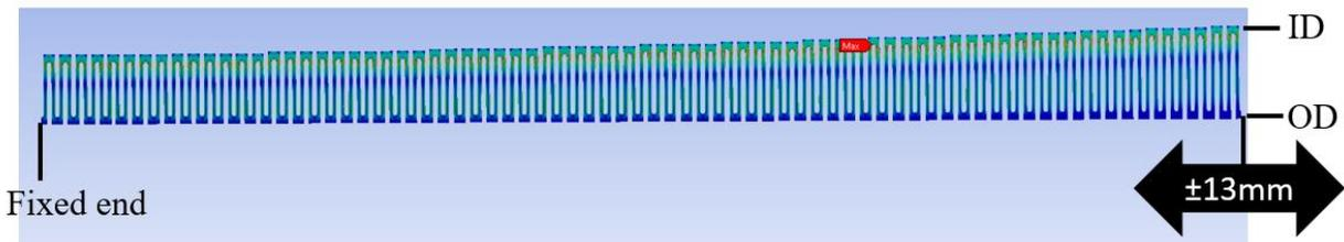
**Fig. 12 Variable ID bellows cross section, dynamic stress distribution at 55 Hz, high stresses in red, low stresses in blue**
