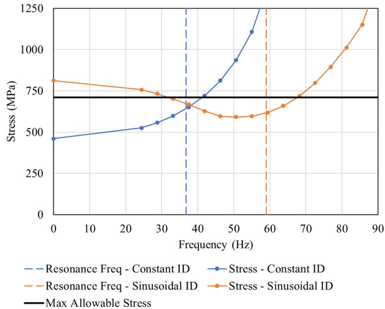
**Fig. 14 Maximum stress vs. frequency for constant and sinusoidal ID – AerMet 100**
