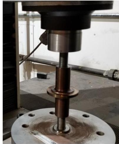
**Fig. 18 Pull test rig**
