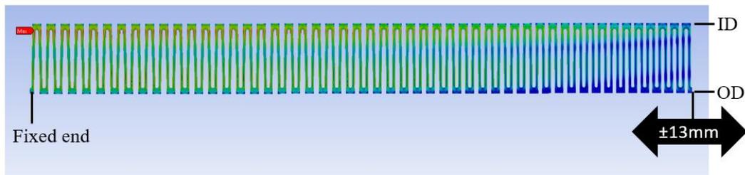
**Fig. 9 Bellows cross section, dynamic stress distribution at 55 Hz, high stresses in red, low stresses in blue**
