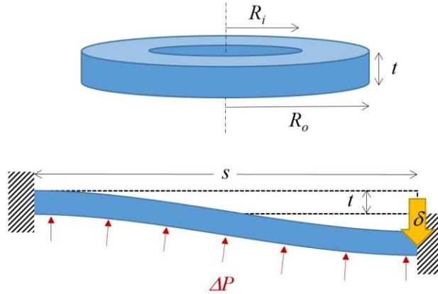
**Fig. 8 Geometry for simple bellows analysis**
