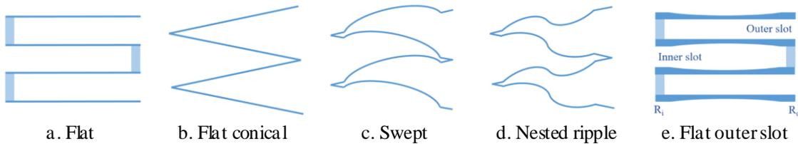
**Fig. 5 Bellows convolution shapes**
