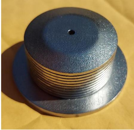
**Fig. 15 3D printed short bellows**
