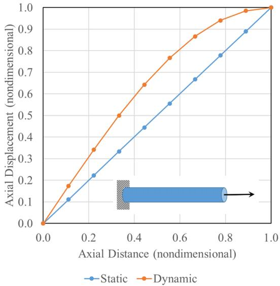
**Fig. 10 Bar axial displacement**
