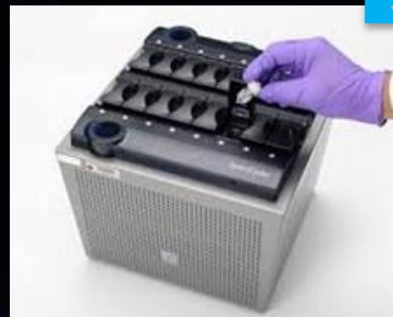
Reaction tube containing lyophilized chemical assay bead (proprietary)
