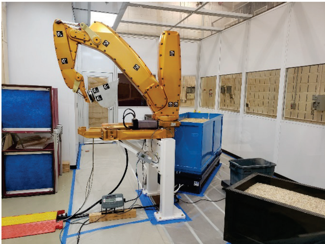
Figure 1. Excavation Lab at NASA Glenn Research Center houses the Advanced Planetary Excavator (APEX) and soil bins inside a dust enclosure.
