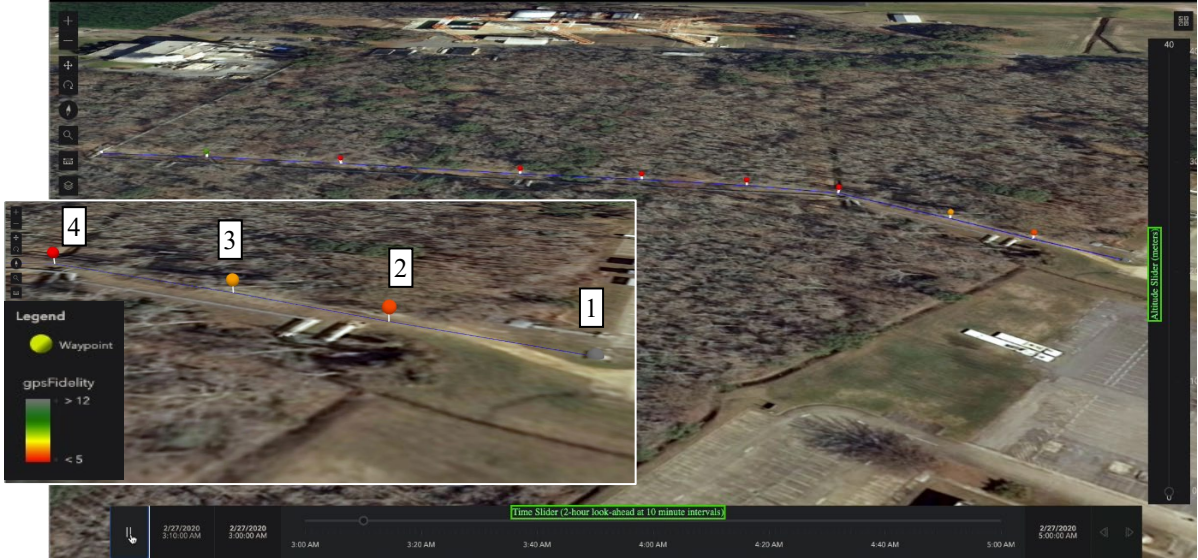
Fig. 5. Forecast of GNSS positioning quality in arboreal canyon. Waypoints along the steam pipeline flight range are raycast to the changing GNSS constellation. The slider at right selects altitude offset from the input flight path and is set to 0 m offset from a ground level input altitude in this image. The slider at bottom selects time in 10 minute intervals. In this forecast, any blockage along the ray is assumed to completely block the satellite. The number of unblocked satellites is tallied and assigned a thermometer color ranging from red to green to grey. Inset: Closeup of the four easternmost waypoints, numbered from east to west. The launch point at right (waypoint 1) receives 12 satellites without attenuation while deep in the canyon at left less than 5 satellites are in clear line of sight. ©Map data: NASA
