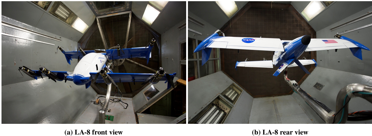
Fig. 1 LA-8 mounted in the NASA Langley 12-Foot Low-Speed Tunnel.
