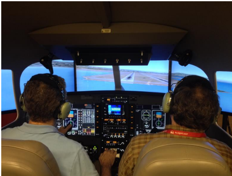
Fig. 4. Interior view of flight simulation test bed for piloted evaluations.
