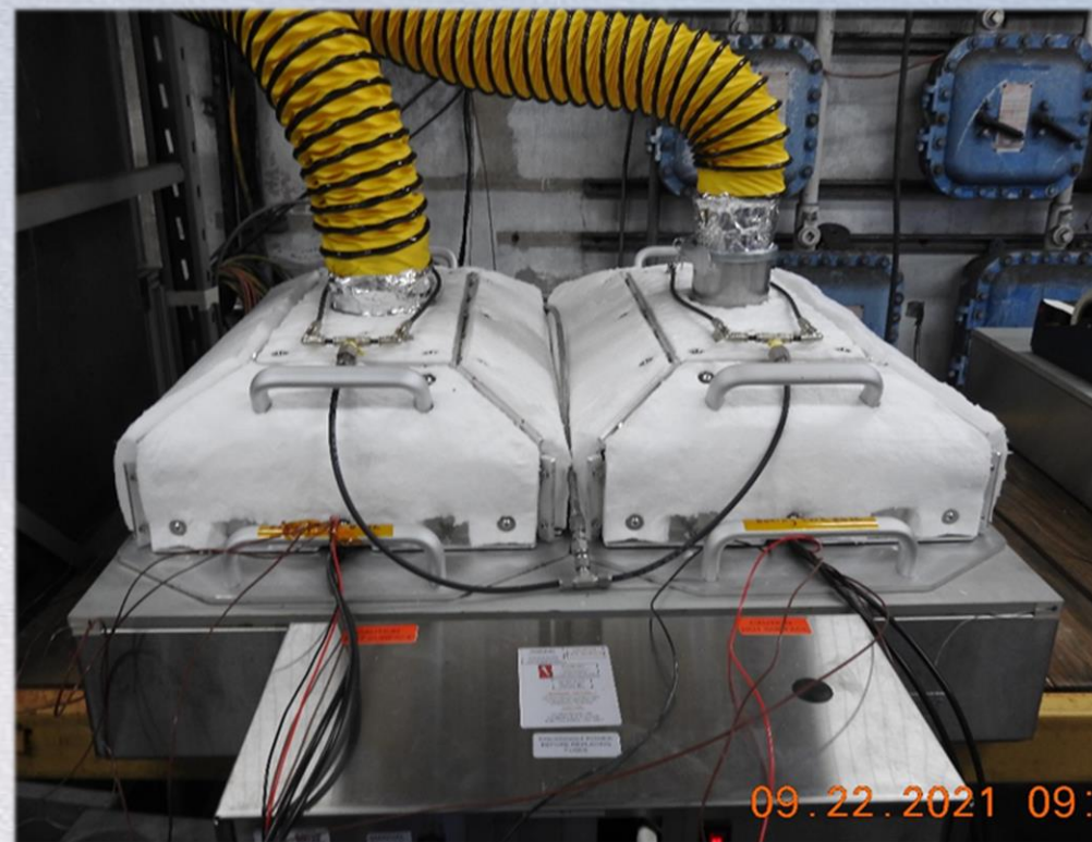
Figure: Battery Design 1 BTA on hot plate prior to heating cells into thermal runaway.
