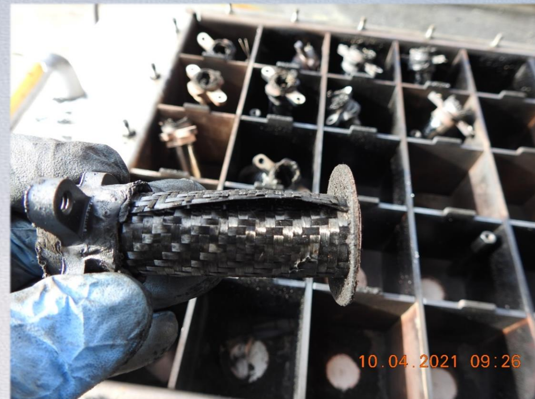
Figure: Panasonic NCRA cell with 0.018" CFT post thermal runaway. Note the thermal abuse sustained by the upper cell support and bursting of the CFT at the seam.
