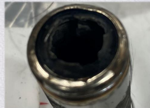
Figures: Cell #18 of BTA 18 – MoliceL INR-18650-M35A Cell with 0.012" CFT after thermal runaway. Note the plastic header burn through. No SWR or SGR observed.
