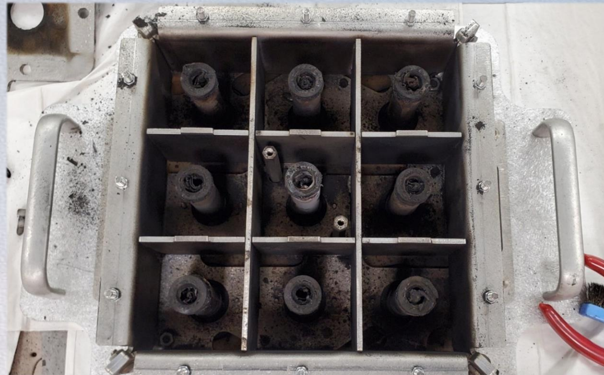
Figure: Battery Design 2 sub-scale BTAs with the upper support plate has been removed. Note that the cells are separated into grid cells to prevent cells from biasing other neighboring cells during thermal runaway. Each cell releases ejecta into its own designated volume which is guarded off from neighboring cell volumes.
