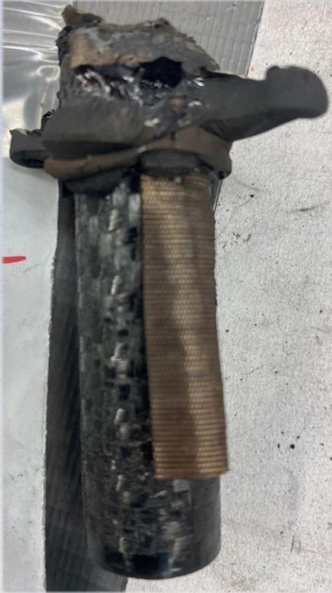
Figures: Cell #12 of BTA 18 – MoliceL INR-18650-M35A Cell with 0.012" CFT after thermal runaway. Note the thermal abuse sustained by the plastic header and header rupture.
