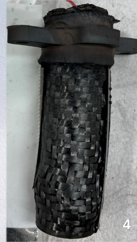
Figures: Cell #44 of BTA 18 – Molicel INR-18650-M35A Cell with 0.012" CFT after TR. Note (1, 2) tiny SGR, but not through plastic header, (5) elongated spin groove on cell with plastic header and CFT removed, (6,7) header rupture.
