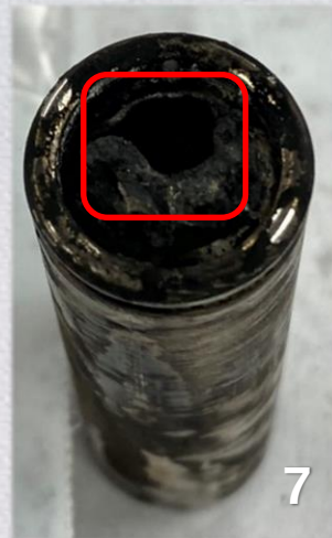
Figures: Cell #44 of BTA 18 – Molicel INR-18650-M35A Cell with 0.012" CFT after TR. Note (1, 2) tiny SGR, but not through plastic header, (5) elongated spin groove on cell with plastic header and CFT removed, (6,7) header rupture.
