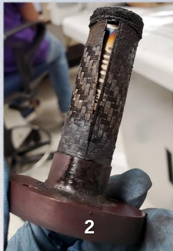
Figures: Molicel INR-18650-M35A cells from Battery Design 2 Sub-Scale BTA after thermal runaway. Note (1) G10/ceramic ring is missing and CFT is mostly in tact but split, (2) G10 is severely burned and CFT is split and burned towards the positive button of the cell, (3) G10 ring burned and CFT split but mostly in tact, (4) large split of CFT. No SWR or SGR identified in 9-cell sub-scale BTA test.
