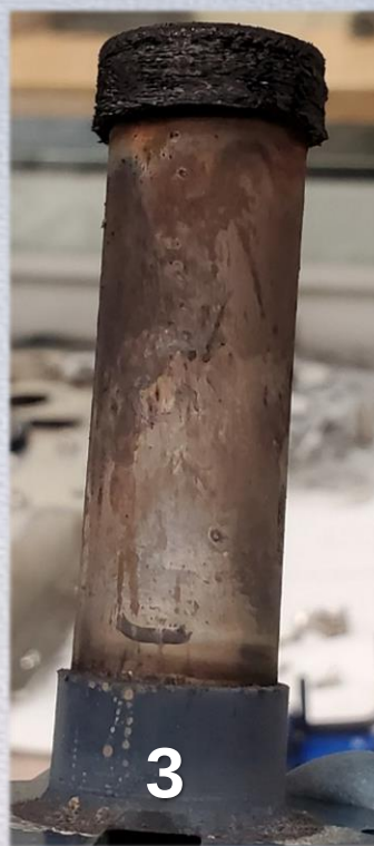
Figures: LG INR18650M36 cells from Battery Design 2 Sub-Scale BTA after thermal runaway. Note (1) header mostly in tact, (2) header completely gone with G10 still connected to the cell, (3) side view of cell with G10 burned, (4) partial jellyroll ejection and (5) G10/ceramic ring missing with top rupture of the cell. No SWR or SGR identified in 9-cell sub-scale BTA test.
