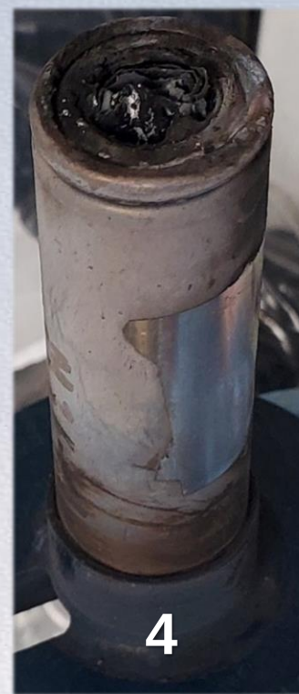
Figures: LG INR18650M36 cells from Battery Design 2 Sub-Scale BTA after thermal runaway. Note (1) header mostly in tact, (2) header completely gone with G10 still connected to the cell, (3) side view of cell with G10 burned, (4) partial jellyroll ejection and (5) G10/ceramic ring missing with top rupture of the cell. No SWR or SGR identified in 9-cell sub-scale BTA test.
