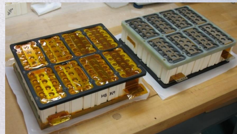
Figure: Four Superbricks connected in 14P-8S comprise single battery pack.
