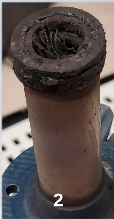
Figures: LG INR18650M36 cells from Battery Design 2 Sub-Scale BTA after thermal runaway. Note (1) header mostly in tact, (2) header completely gone with G10 still connected to the cell, (3) side view of cell with G10 burned, (4) partial jellyroll ejection and (5) G10/ceramic ring missing with top rupture of the cell. No SWR or SGR identified in 9-cell sub-scale BTA test.
