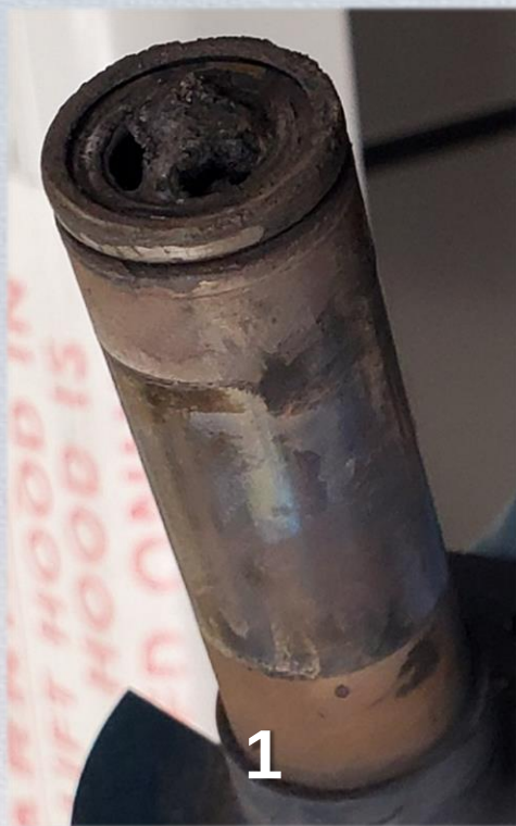
Figures: LG INR18650M36 cells from Battery Design 2 Sub-Scale BTA after thermal runaway. Note (1) header mostly in tact, (2) header completely gone with G10 still connected to the cell, (3) side view of cell with G10 burned, (4) partial jellyroll ejection and (5) G10/ceramic ring missing with top rupture of the cell. No SWR or SGR identified in 9-cell sub-scale BTA test.
