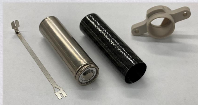
Figure: LG M36 cell with 0.012" CFT.
