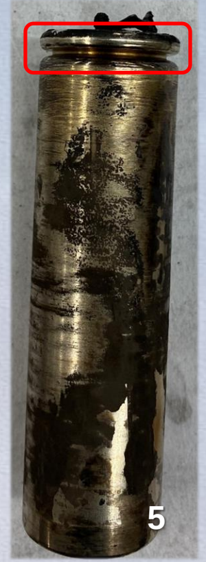
Figures: Cell #44 of BTA 18 – Molicel INR-18650-M35A Cell with 0.012" CFT after TR. Note (1, 2) tiny SGR, but not through plastic header, (5) elongated spin groove on cell with plastic header and CFT removed, (6,7) header rupture.
