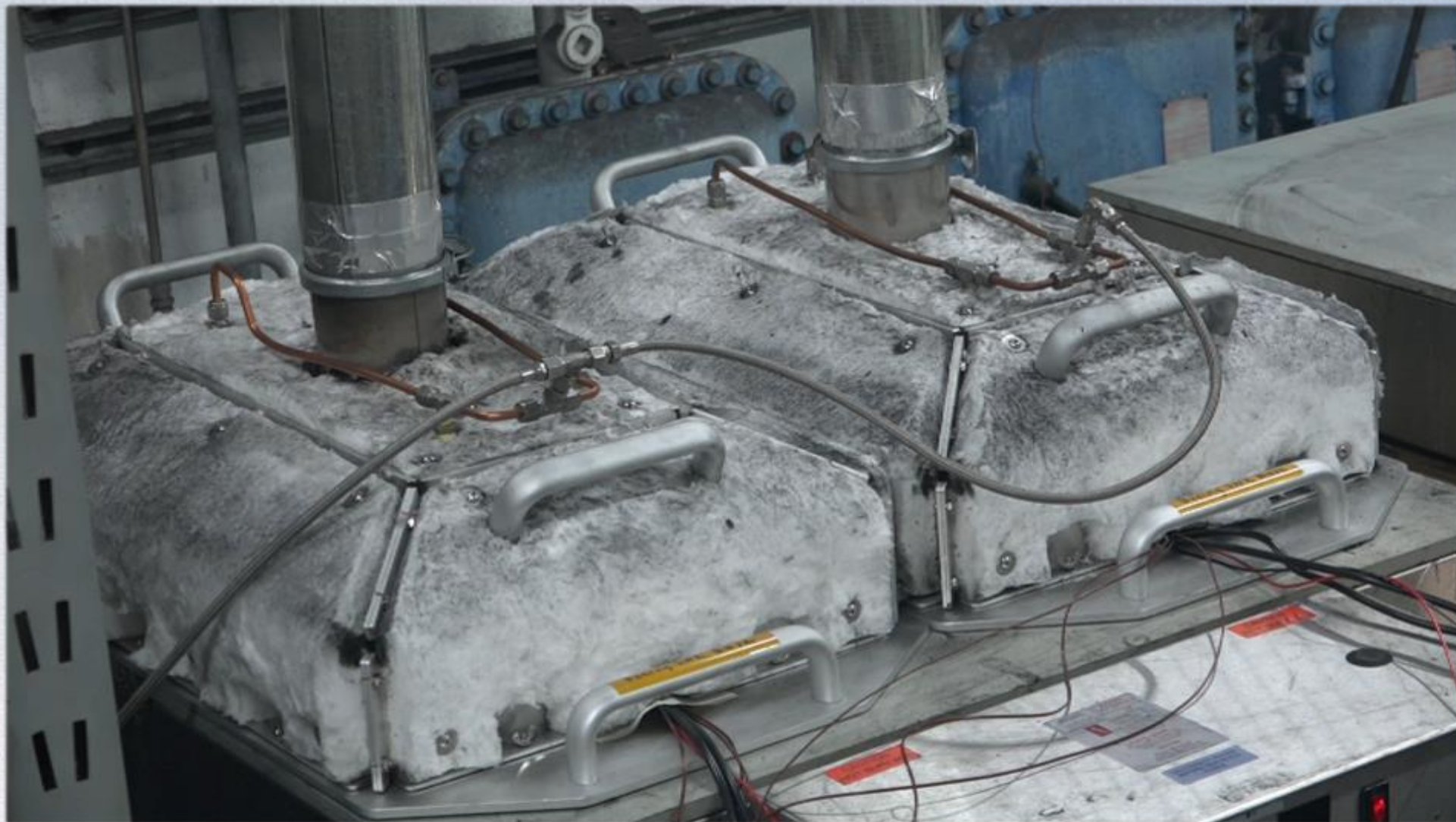
Battery Design 1 Side Wall Rupture Test Run 2 of LG M36 Bare Cells (9/23/2021)
