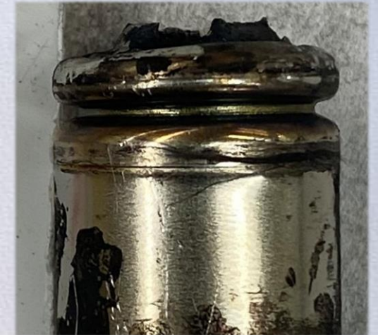
Figures: Cell #18 of BTA 18 – MoliceL INR-18650-M35A Cell with 0.012" CFT after thermal runaway. Note the plastic header burn through. No SWR or SGR observed.
