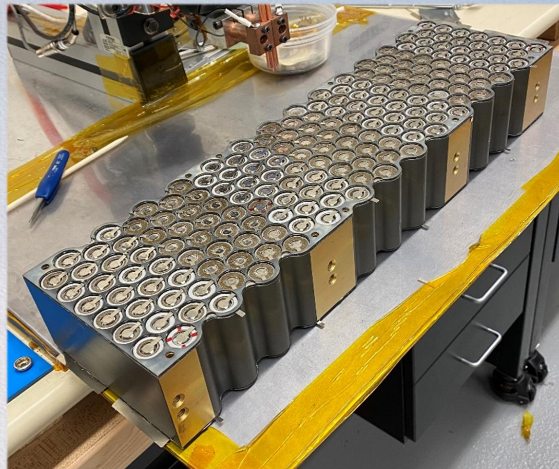
Figure: Battery Design 3 with an interstitial aluminum heat sink with cells spaced 0.020" apart (156 cell heat sink).
