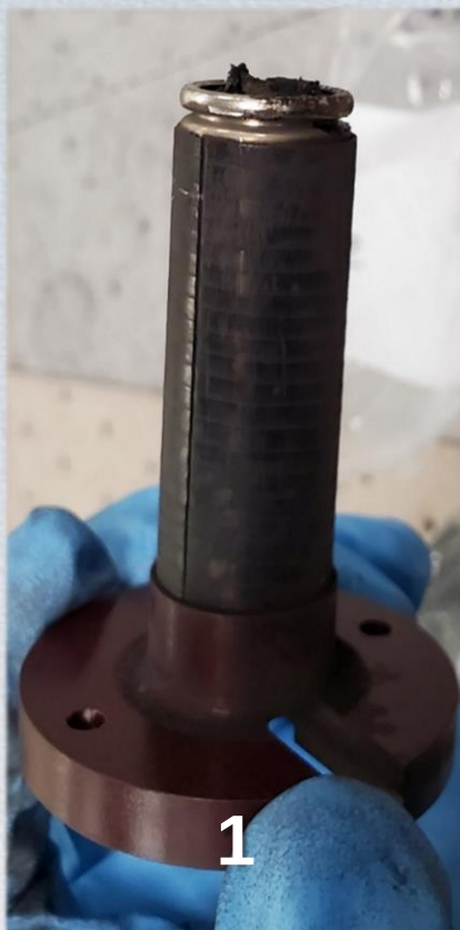
Figures: Molicel INR-18650-M35A cells from Battery Design 2 Sub-Scale BTA after thermal runaway. Note (1) G10/ceramic ring is missing and CFT is mostly in tact but split, (2) G10 is severely burned and CFT is split and burned towards the positive button of the cell, (3) G10 ring burned and CFT split but mostly in tact, (4) large split of CFT. No SWR or SGR identified in 9-cell sub-scale BTA test.
