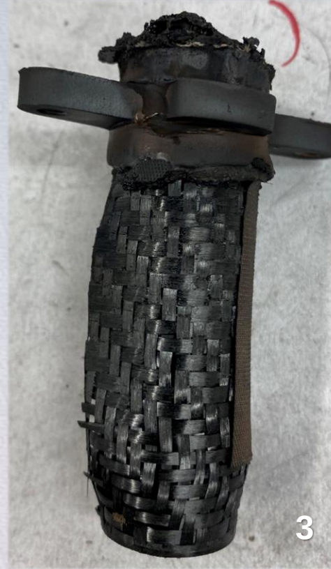
Figures: Cell #44 of BTA 18 – Molicel INR-18650-M35A Cell with 0.012" CFT after TR. Note (1, 2) tiny SGR, but not through plastic header, (5) elongated spin groove on cell with plastic header and CFT removed, (6,7) header rupture.
