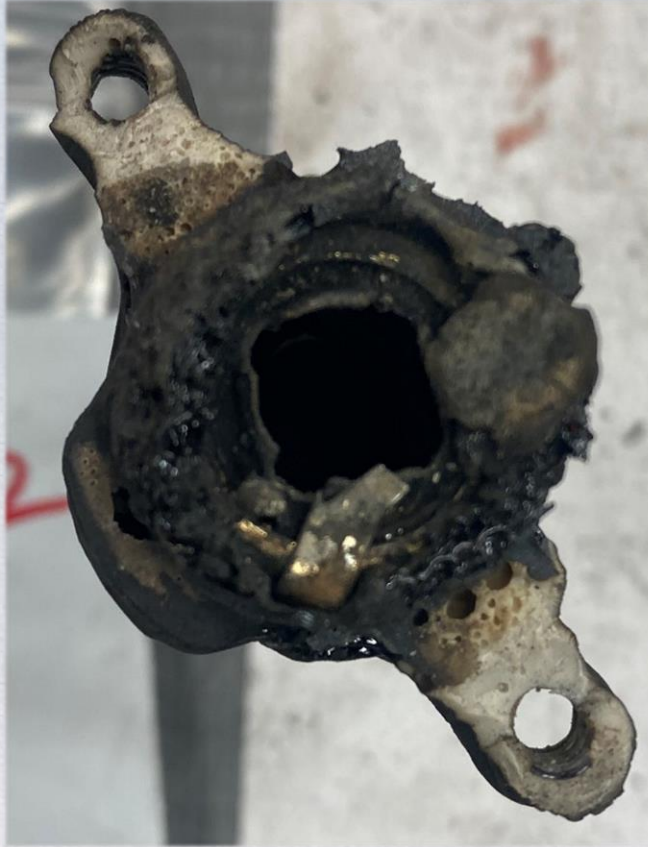
Figures: Cell #12 of BTA 18 – MoliceL INR-18650-M35A Cell with 0.012" CFT after thermal runaway. Note the thermal abuse sustained by the plastic header and header rupture.
