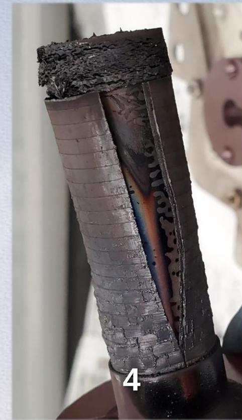
Figures: Molicel INR-18650-M35A cells from Battery Design 2 Sub-Scale BTA after thermal runaway. Note (1) G10/ceramic ring is missing and CFT is mostly in tact but split, (2) G10 is severely burned and CFT is split and burned towards the positive button of the cell, (3) G10 ring burned and CFT split but mostly in tact, (4) large split of CFT. No SWR or SGR identified in 9-cell sub-scale BTA test.
