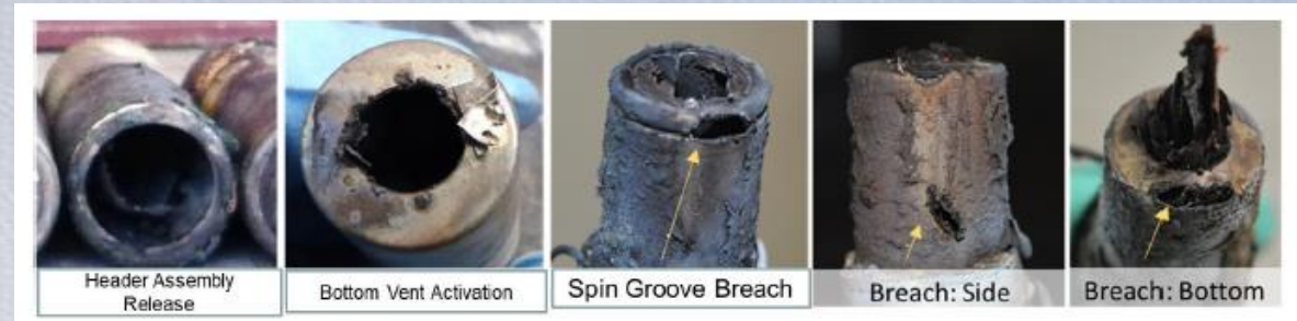
Figure: Examples of common cell failure modes after thermal runaway.
