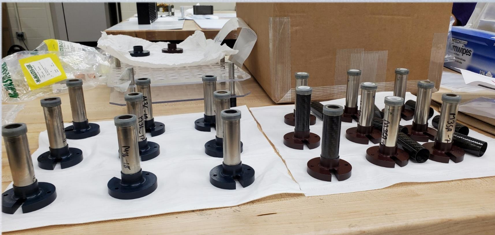
Figure: Two cell configurations (1) bare LG INR18650M36 cells (no sleeve support) along with (2) Molicel INR-18650-M35A with 0.012" thick CFT prepared for testing. The CFT was manufactured in two layers: 1 st layer ~0.0035" thick unidirectional, 2 nd layer ~0.008" thick 2x2 twill. The two cells above were tested to compare against incumbent Panasonic NCR18650B cell design.
