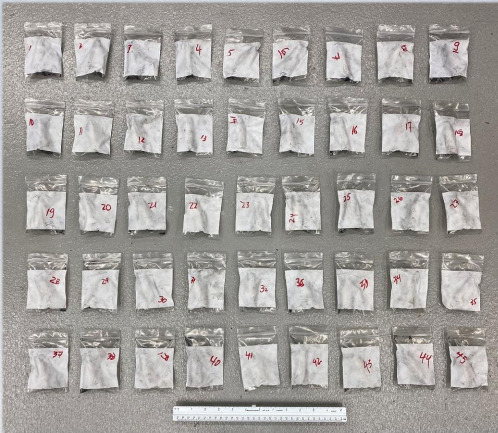
Figure: Cells were bagged and serialized post test to keep ejecta with each cell for a more detailed examination.
