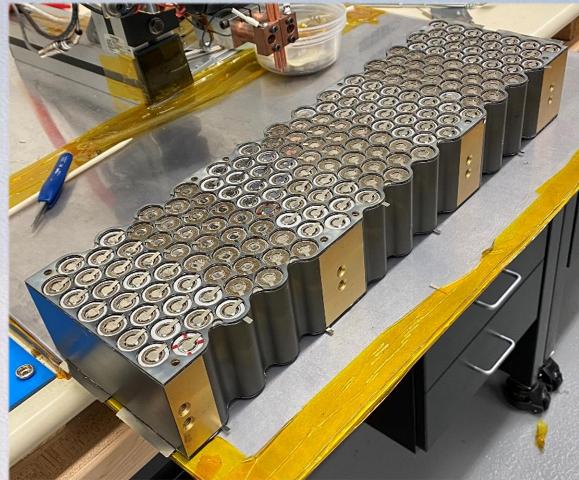
Figure: Battery Design 3 with an interstitial aluminum heat sink with cells spaced 0.020" apart (156 cell heat sink).
