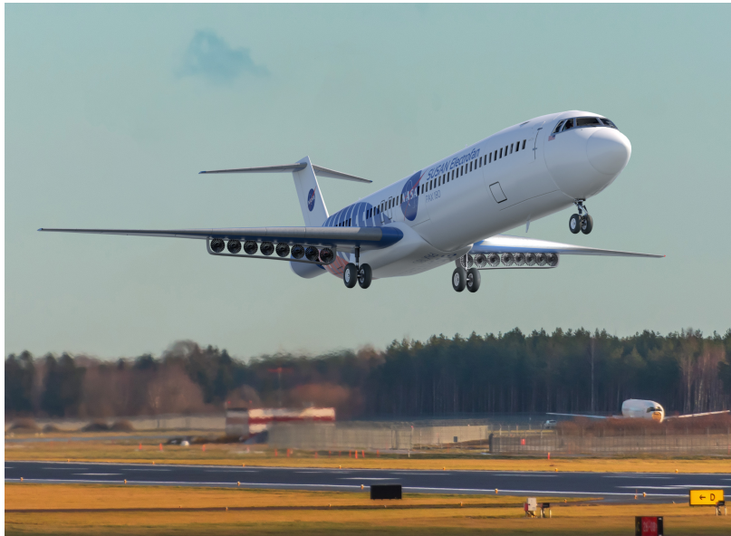
Fig. 1 An artist's rendering of the SUSAN Electrofan concept, illustrating the T-tail, single aft turbofan, and the wing-mounted electric engines.
