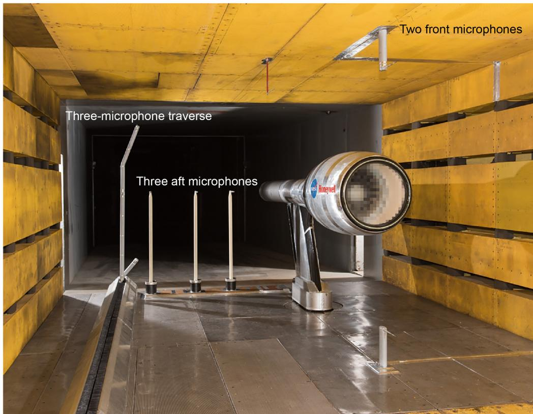
Figure 87.—Forward looking aft at 9 by 15-Foot Low-Speed Wind Tunnel test section with representative model and microphones, 1986 configuration. Test section support frame is visible in slots, covered with foam.
