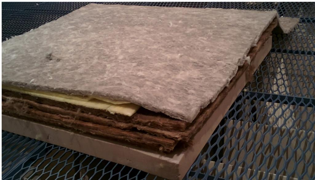
Figure 71.—Stack of batted fiber bulk absorbers over steel sheet placed on top of piece of gray melamine foam.
