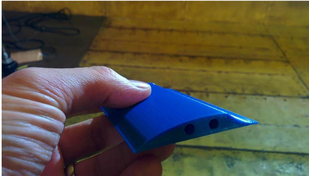
Figure 36.—Segment of two-dimensional linear hump geometry used to create modified boundary layer on wall of roughness noise facility at Virginia Polytechnic Institute and State University.
