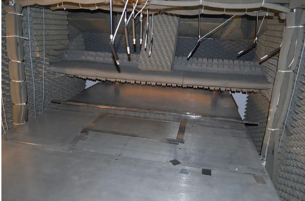
Figure 37.—Virginia Polytechnic Institute and State University roughness noise facility with cross-stream linear bump installed upstream of test sample.
