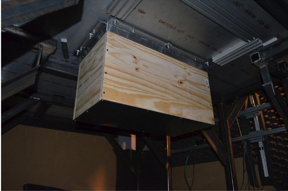
Figure 19.—View of acoustic absorber box installed below wall jet facility at Virginia Polytechnic Institute and State University. Photograph taken June 2, 2014.
