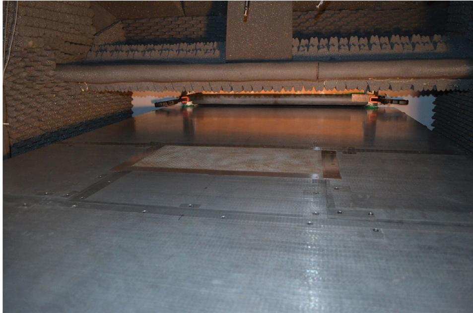
Figure 21.—Flush mount installation showing panel size. Facility can also accept panels up to 61 by 61 cm (2 by 2 ft), as this figure illustrates. Fasteners visible are covered with clear piece of thin packing tape. Test sample edges are treated with aluminum tape.
