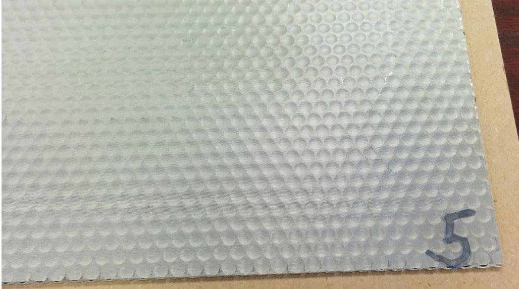
Figure 35.—Diffusion bonded panel 5 showing dimpling of approximately 0.18-mm (0.007-in.) depth.
