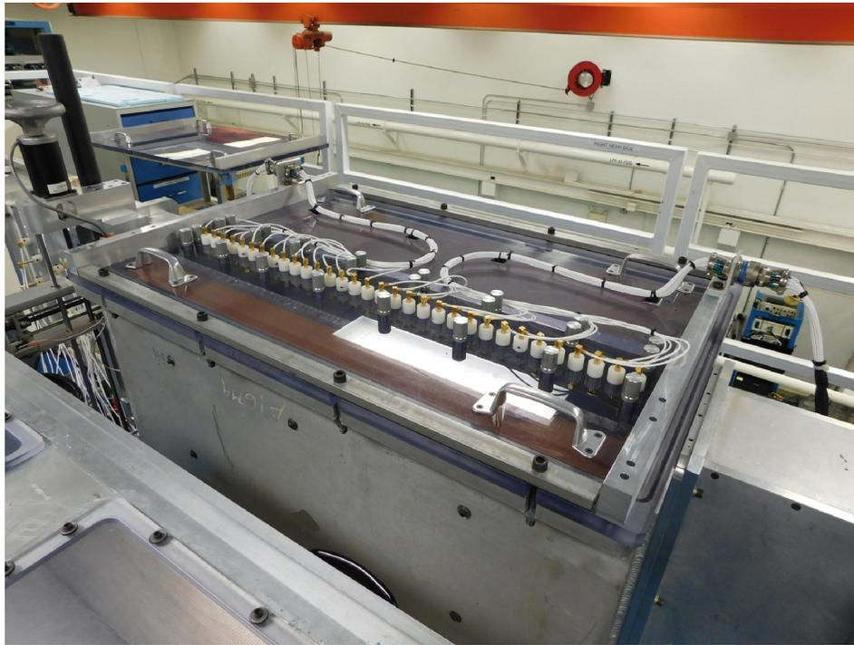
Figure 84.—Sample ready to test at NASA Langley Research Center facility. Flow is from right to left.
