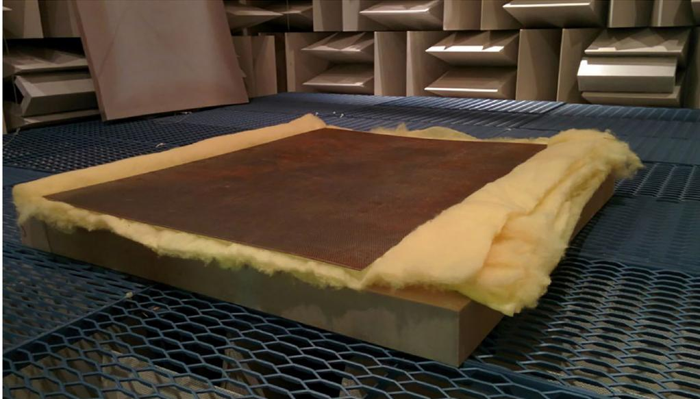
Figure 69.—Simulated 1986 acoustic treatment used over beams.
