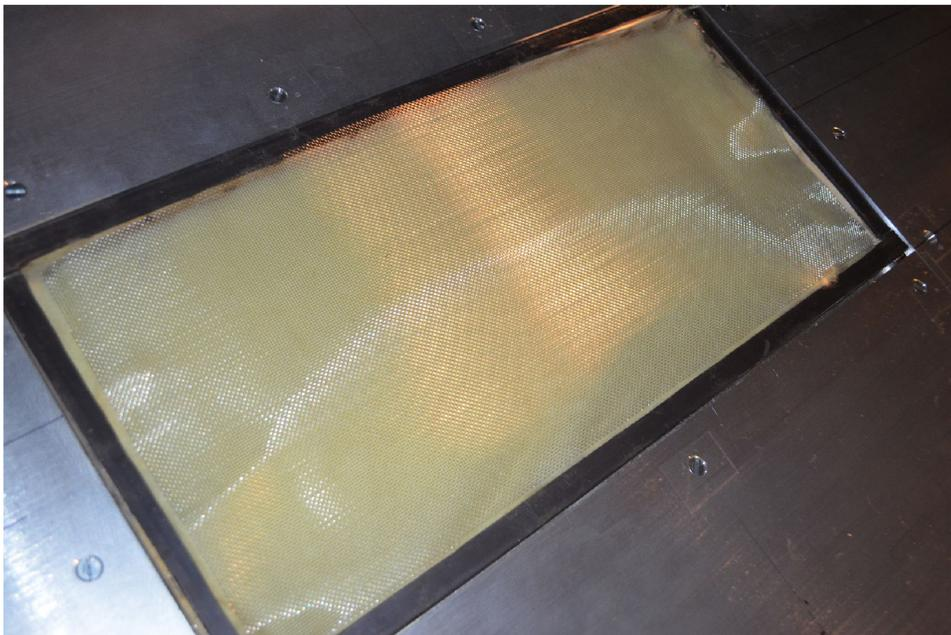
Figure 20.—Top view of Kevlar® (DuPont™) treatment inside acoustic box, mesh (20 wires per inch) screen on top. Perforate plate flow surface and tape for edges yet to be applied.
