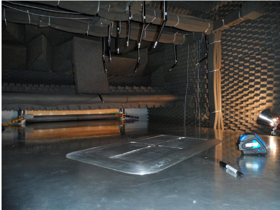
Figure 10.—Frame used for Virginia Polytechnic Institute and State University testing, without sample installed.
