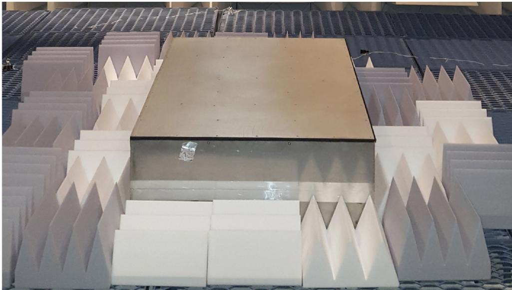
Figure 77.—Prototype acoustic box tested in NASA Glenn Research Center Acoustical Testing Laboratory in December 2017.
