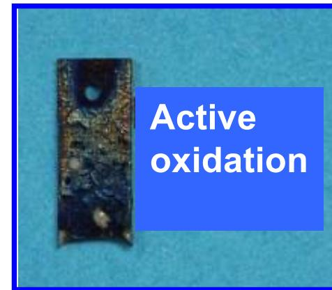
Transition between passive and active oxidation regimes depends on temperature and partial pressure of oxygen
