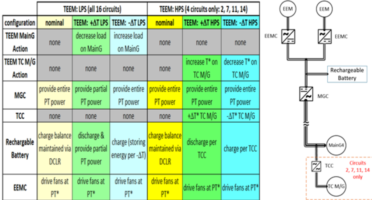
Figure 3: SUSAN EPS TEEM Implementation, with Single Bus Schematic
