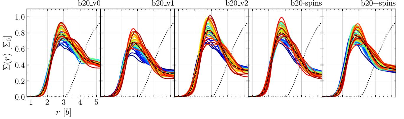
**Figure 13.** Vertically integrated and  $\phi$ -averaged density  $\Sigma(r)$  averaged over  $\Delta t = 2 \times 10^3 M$  for the period  $t = 70 - 150 \times 10^3 M$  (violet to red curves). The dotted curve represents the initial data, and the dashed curve the average of colored curves.
