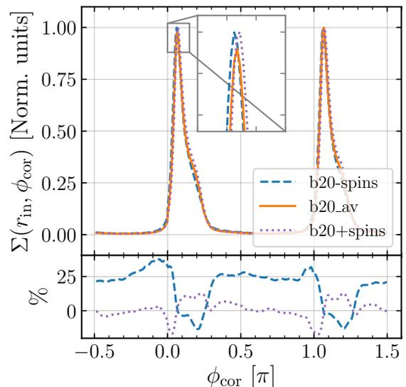
**Figure 8.** *Top:* Surface density, averaged during the steady state period, in the corotating frame of the binary, and evaluated at the radial inner boundary of the domain  $r_{\text{in}}$ , for spinning runs and the average of non-spinning runs (**b20\_av**). *Bottom:* Percent deviation of curves for spinning runs with respect to the non-spinning average.
