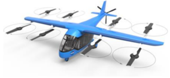
(b) NASA Lift-Plus-Cruise Vehicle Schematic (credit: NASA Langley Research Center)
